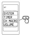
"CH MACRO" appears on the LCD display, and component names are displayed on the labels.
